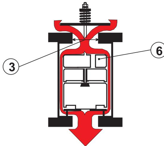
Upon pump stop, the pump discharge check valve closes. Liquid drains from the air valve and the pump's vertical column. The negative differential created by the draining liquid causes atmospheric air to push the "Anti-Shock" Float (6) down, opening the Large Orifice (3) and rapidly displaces the draining liquid to prevent potentially damaging internal negative pressure\*.
