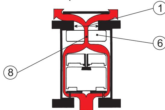
In reaction to increased air flow, Float (6) closes Large Orifice (1) and air is forced through the “Anti-Shock” Orifice (8) resulting in deceleration of the approaching water due to the resistance of rising air pressure in the valve.
