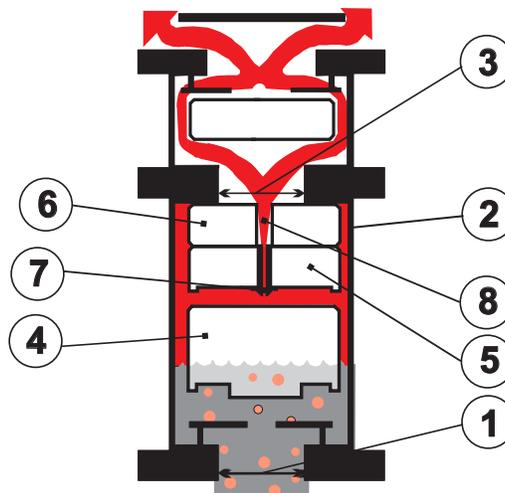
Subsequent to the filling of a pipeline, liquid enters the valve Barrel Chamber (2) and the Floats (4), (5) and (6) are buoyed so that the "Anti-Shock" Orifice (8) is closed by the Float (5) and the valve will then become pressurized. A minimal working pressure of <math><0.5\text{ bar (7.3 psi)}</math> acting on a relatively large area of the Orifice (1) will lock Floats (5) and (6) into the closed position across the Large Orifice (3).
