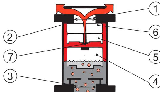
Subsequent to the filling of a pipeline, liquid enters the valve Barrel Chamber (2) and the Floats (4), (5) and (6) are buoyed so that the Large Orifice (1) is closed by Float (6), the valve will then become internally pressurized. A minimal working pressure of < 0.5 bar (7.3 psi) acting on the relatively large area of the Orifice (1) will lock Float (6) into the closed position across the Large Orifice (1).
