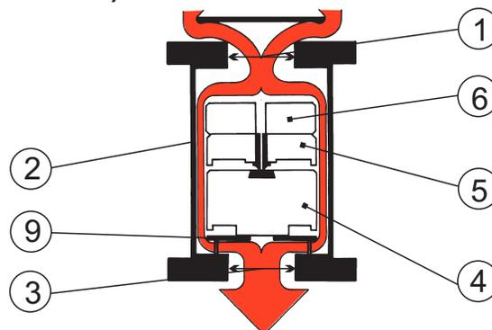
Simultaneous drainage of liquid from Valve Chamber (2) causes Floats (4), (5) and (6) to gravitate downwards onto the Baffle Plate (9), thereby allowing atmospheric air through the valve to rapidly displace draining liquid in the pipeline and prevent potentially damaging internal negative pressure.
