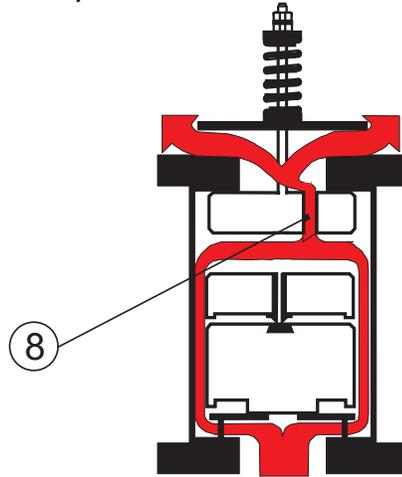
Air is forced through the "Anti-Shock" Orifice (8) resulting in the deceleration of the approaching water column due to the resistance of rising air pressure in the valve. This dampens transients when the air valve closes and the water column opens the pump, discharge check valve.
