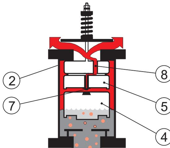
Liquid enters the valve Barrel Chamber (2) and the Floats (4), (5) are buoyed so that the "Anti-Shock" Orifice (8) is closed by the Floats (4), (5) the valve will then become internally pressurized.
